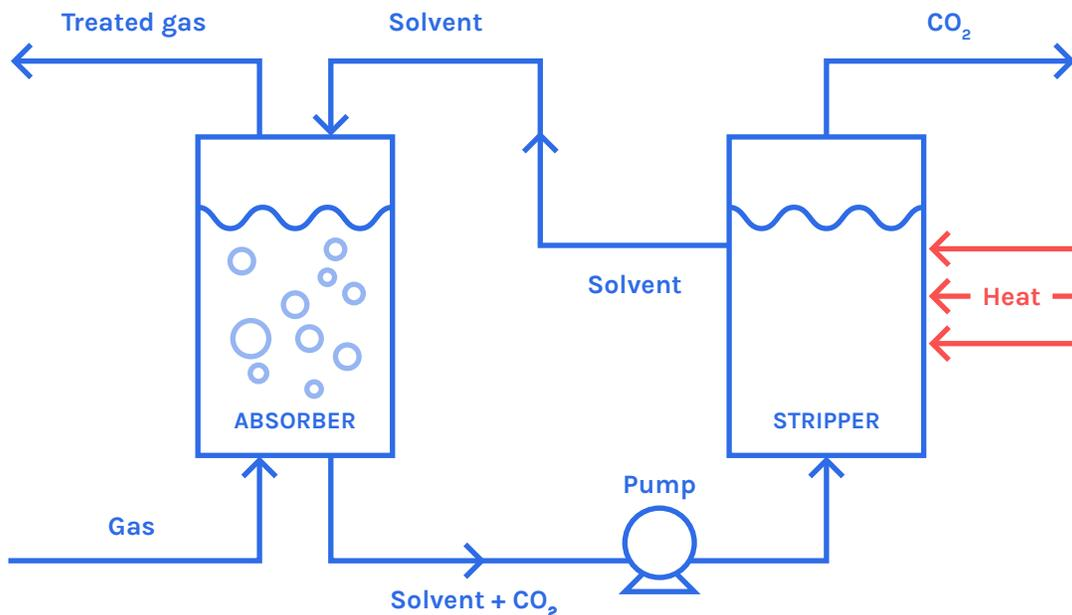
Basic overview of a liquid absorption process
