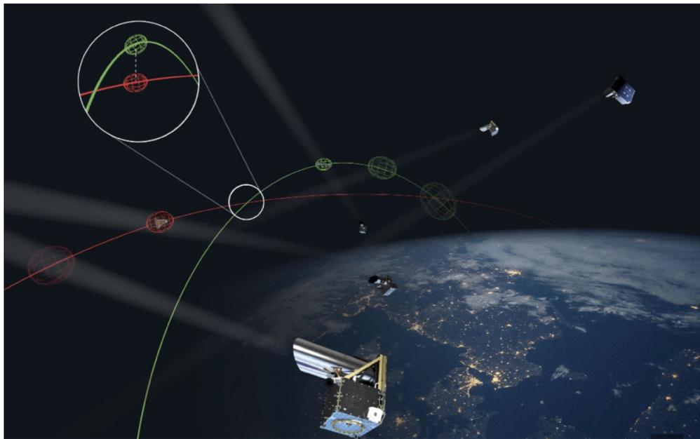
*Northstar's constellation of satellites will use optical sensors for tracking objects across multiple orbits.
