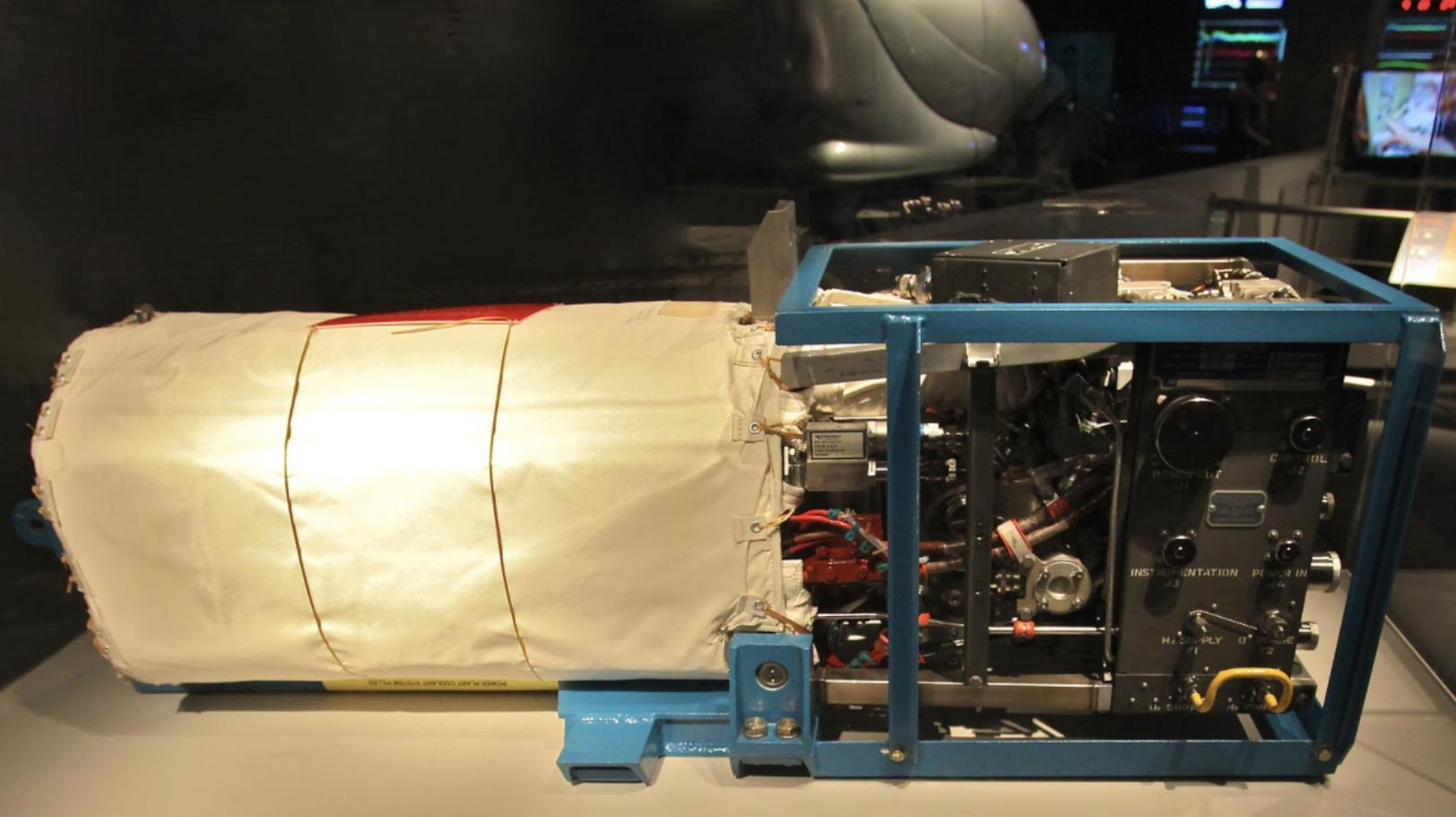
*A fuel cell assembly from the Space Shuttle Orbiter, retired in 2012. So analog!*
