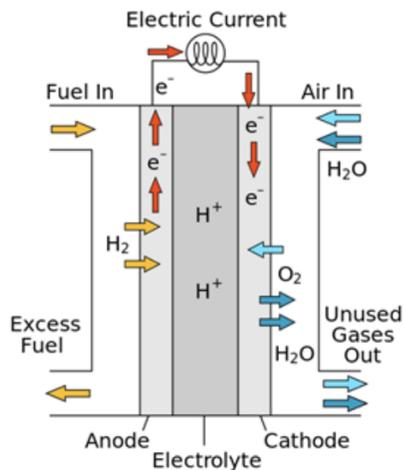
Protons (H<sup>+</sup>) cross the electrolyte to the cathode
