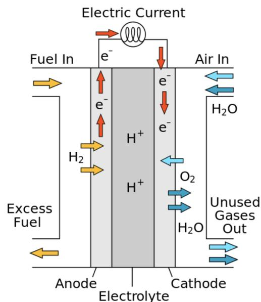
Schematic for a typical PEM fuel cell used in vehicle applications. ([Image Source](#))
