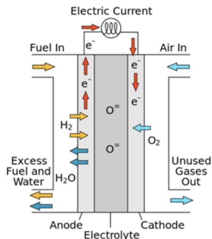
Oxygen ions (O<sup>2-</sup>) cross the electrolyte to the anode
