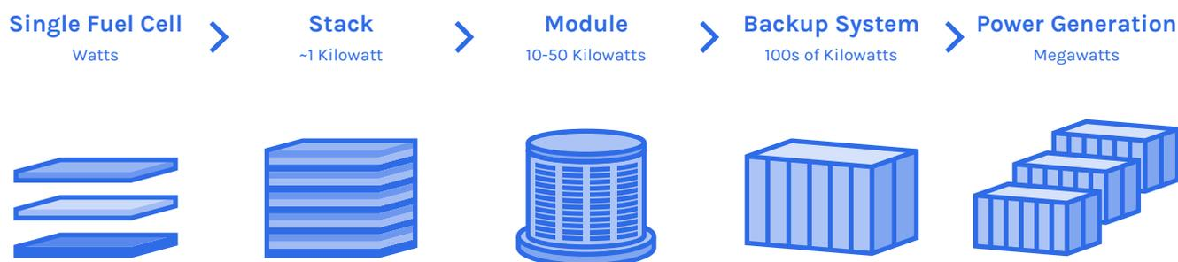
*Individual fuel cells are coupled into stacks to make larger systems. In batteries, leads (wires) are attached to the electrodes in each cell. Fuel cell engineers have a more difficult challenge: they have to design systems to deliver hydrogen and oxygen gases to each cell in the system.*
